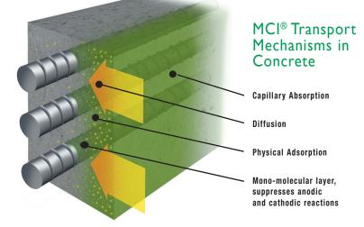
MCI<sup>®</sup> concentration increases with time, showing that the MCI<sup>®</sup> diffuses through the concrete (Figure 2). Using experimentally obtained data, the coefficient of diffusion was calculated (Figure 3 and Table 2). This data demonstrates the migratory nature of MCIs and proves that they can be used for protection against chloride induced corrosion and carbonation.
