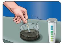
Use the manufacturer's instructions for the EM Quant QAC test sticks to analyze each slurry solution/extraction.
